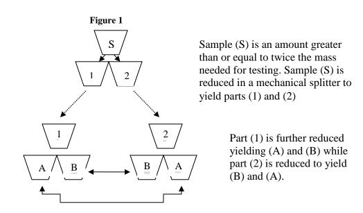
Final testing sample is produced by combining alternate pans, i.e. A/A or B/B only.
